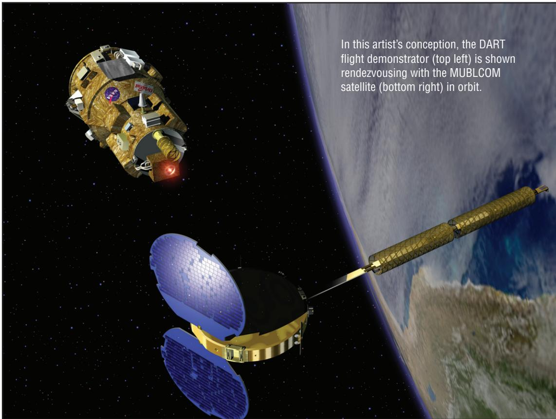
The Demonstration of Autonomous Rendezvous Technology (DART) is a flight demonstrator that provides a key step in establishing autonomous rendezvous capabilities for the U.S. space program. While previous rendezvous and docking efforts have been piloted by astronauts, the unmanned DART spacecraft will have computers and sensors to perform all of its rendezvous functions.
